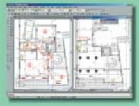
**Automatic Receptor Installation:** FINE/AutoFINE expert automatically installs on the ground plan radiators, fan coils, airduct grills as well as illuminants and switches etc. Moreover, this procedure follows expert intelligence rules, which are open to the
